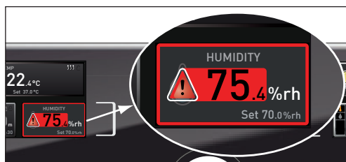
Fig. 22 Humidity monitoring triggered
