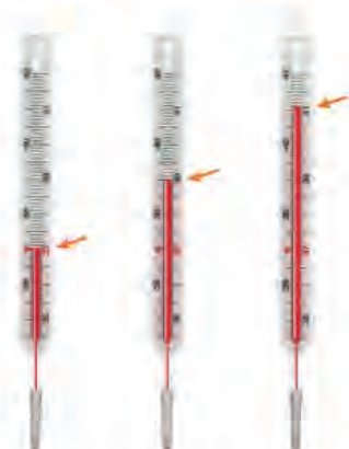
When the temperature increases, the alcohol expands to take up more space.
